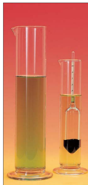
HT400/412 with Hydrometer in use
